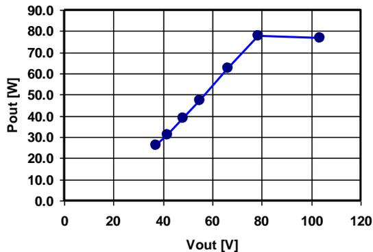
Figure. 6. Measured output P-V behavior with solar cell input power to boost converter.
