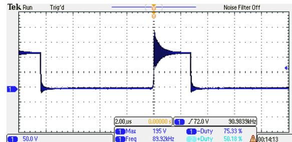
Figure 2. Measured  $V_{ds}$  at 90 kHz switching frequency.  $V_{ds}$  is seen to be switching between about 120V and 0V. The peak voltage is 195V due to ringing when the mosfet turns off.
