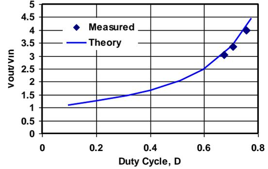
Figure. 4. Measured versus theoretical comparison of  $V_{out}/V_{in}$  ratio as a function of duty cycle  $D$  at a frequency of 30 kHz.
