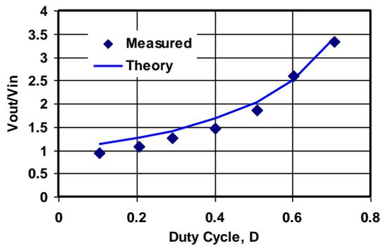
Figure. 5. Measured versus theoretical comparison of  $V_{out}/V_{in}$  ratio as a function of duty cycle  $D$  at a frequency of 90 kHz with solar cell input to boost converter.
