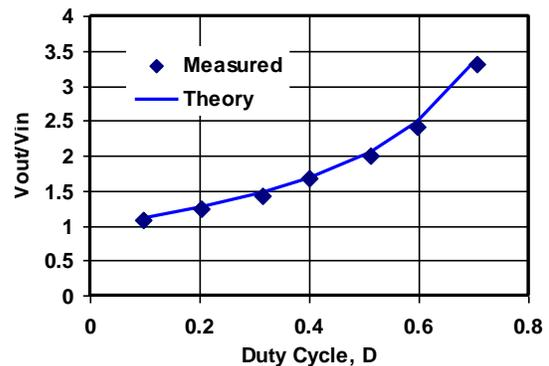
Figure 3. Measured versus theoretical comparison of  $V_{out}/V_{in}$  ratio as a function of duty cycle  $D$  at a frequency of 90 kHz.
